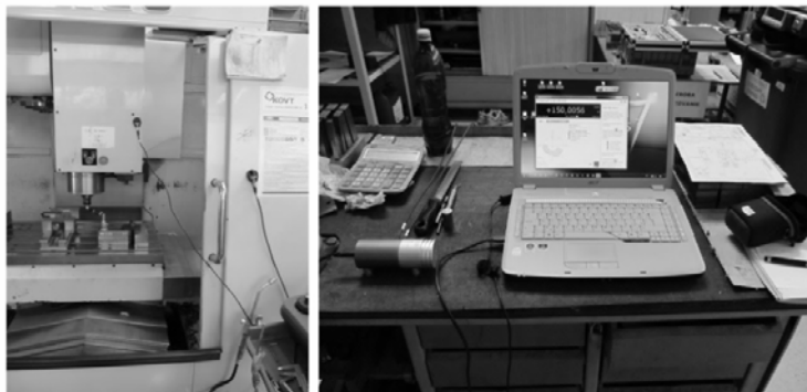
Fig. 2. Measurement of environmental conditions using compensatory unit of equipment Laser XL 80
